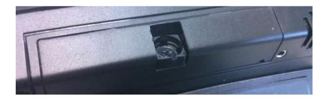
3. Remove the screw, and then detach the cover; this will show the SIM cards and USB port:
