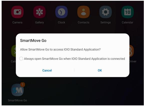
Select the "always open" option, then press OK. Sometimes the Android operating system will skip past this checkbox as it appears, but it is imperative that it gets selected and confirmed, otherwise the IOIO box will be unable to communicate with the SmartMove Go app.
